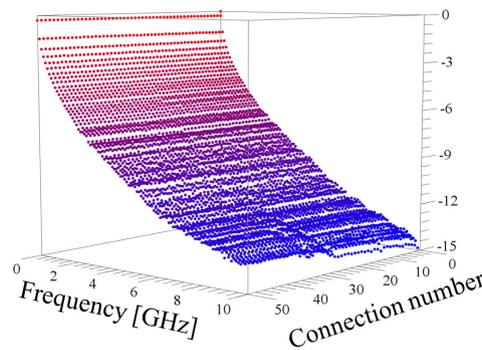
Round trip RF attenuation as a function of connector mating cycle number
