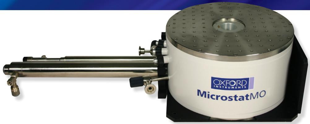
The **MicrostatMO** is a compact stable cryostat, which provides a cryogenic environment (6 K) ideal for sensitive optical and electrical measurements in
