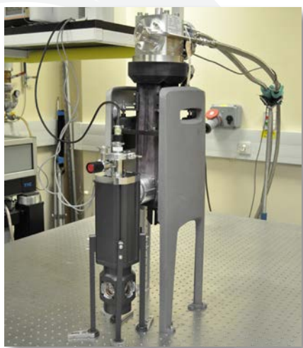
Figure 1. OptistatDry top-loading Cryofree
