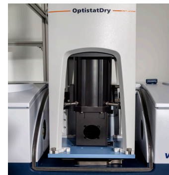
Figure 1. OptistatDry mounted in a Bruker V70 FTIR spectrometer.
