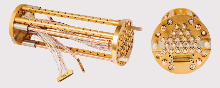
**Improved sample throughput** with our bottom loading mechanism which allows you to get your research up and running quickly, **maximising uptime and efficiency**. Design features include: a short **software-automated cooldown** of only **8 hours**; sample exchange while the system is cold; and no need to worry about warming up the system to remove shields between experiments.
