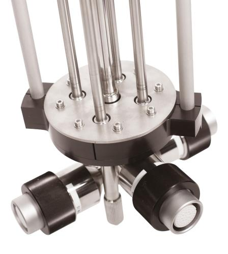
Our patented bottom loader and active gas gap heat switch technology enable fast turnaround times, particularly suited to magnet systems and qubit and device screening.
