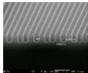
GaAs/AlGaAs photonic cavity etch
