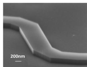
Etched strip waveguide on SOI with clean and smooth sidewall for low propagation loss
