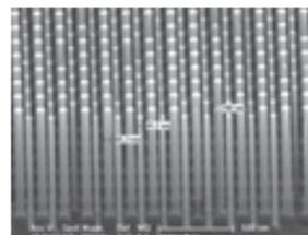
Deep Si etch nanowires formed from dense 40 & 60 nm pillars
