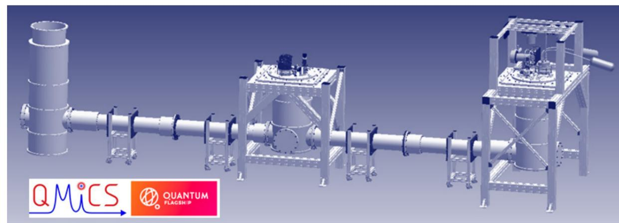
Design model of quantum teleportation system between two superconducting quantum devices operating below 50 mK with inter-fridge communication circuit also held at mK temperatures along its length.
