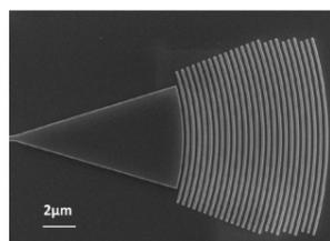
Etched grating coupler and taper waveguide on SOI
