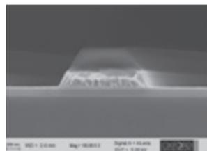
300 nm Nb etched to SiO<sub>2</sub> for superconducting electronics
