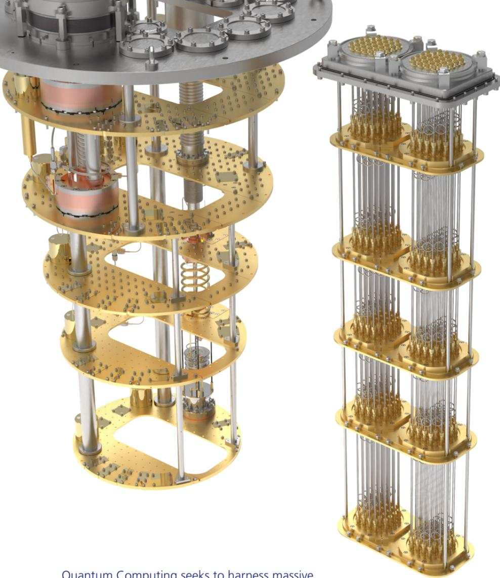
High performance closed-cycle coolers enable cryogen free mK temperatures to be readily achieved with large sample volumes, high cooling powers and significant wiring assemblies for high line count applications such as quantum computing.
