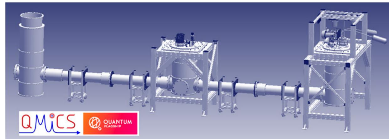
Design model of quantum teleportation system between two superconducting quantum devices operating below 50 mK with inter-fridge communication circuit also held at mK temperatures along its length.
