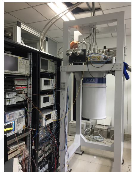
Experimental set-up with Triton 500 Cryofree dilution refrigerator
