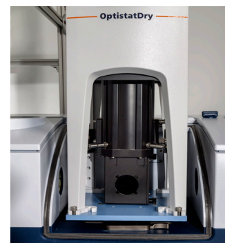
Figure 1. OptistatDry mounted in a Bruker V70 FTIR spectrometer.
