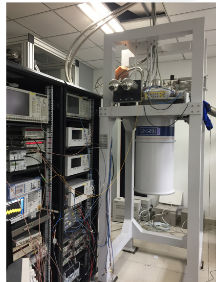
Experimental set-up with Triton 500 Cryofree dilution refrigerator
